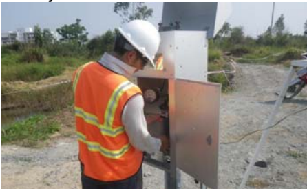
Sampling air to ensure contamination does not leave Project site (Photo: CDM Smith)
